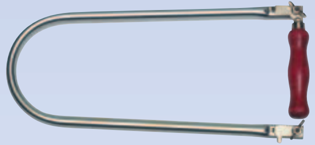
Art. 710 Stahlrohr 13 mm, vernickelt, 320 mm Ausladung, Spezial-Spannplättchen, Stahlflügelmuttern Art. 710 Tubular steel 13 mm, nickel-plated, throat depth 320 mm, with special tension plates, steel wing nuts
