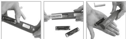
**Inserting the batteries:** The electrical drill uses two 1,5V batteries (AA). Slide off the cover (4) at the end of the drill to open the battery compartment; insert the 2 batteries, the + pole towards the front end of the drill. Slide back the cover.
